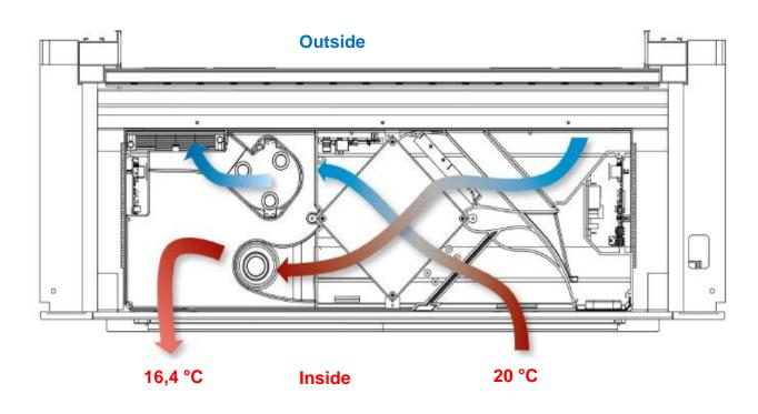
Due to the «Enthalpy» heat exchanger there is no need to provide water drainage system
