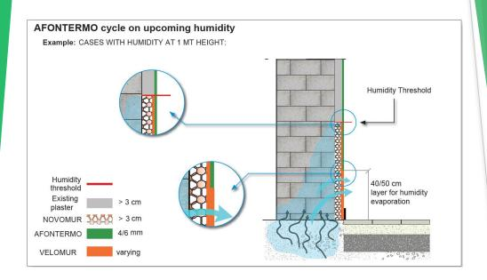
**VELOMUR®** is used for surface finishing and/or thermal insulation. It is highly breathable, specifically designed to complete the thermo-depressurizing cycle of **NOVOMUR®** plaster.
