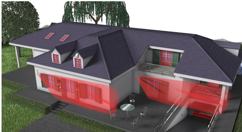
External peripheral protection (doors and windows) by Active Infrared Beareers (Winbeam / Doorbeam) and Passive Infrared Detectors (Tried).
